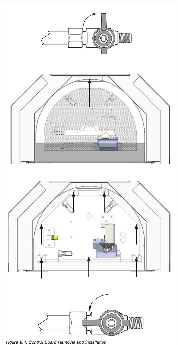
Figure 8.4, Control Board Removal and Installation
