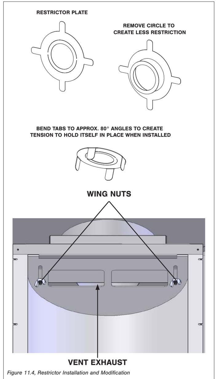
Figure 11.4, Restrictor Installation and Modification
