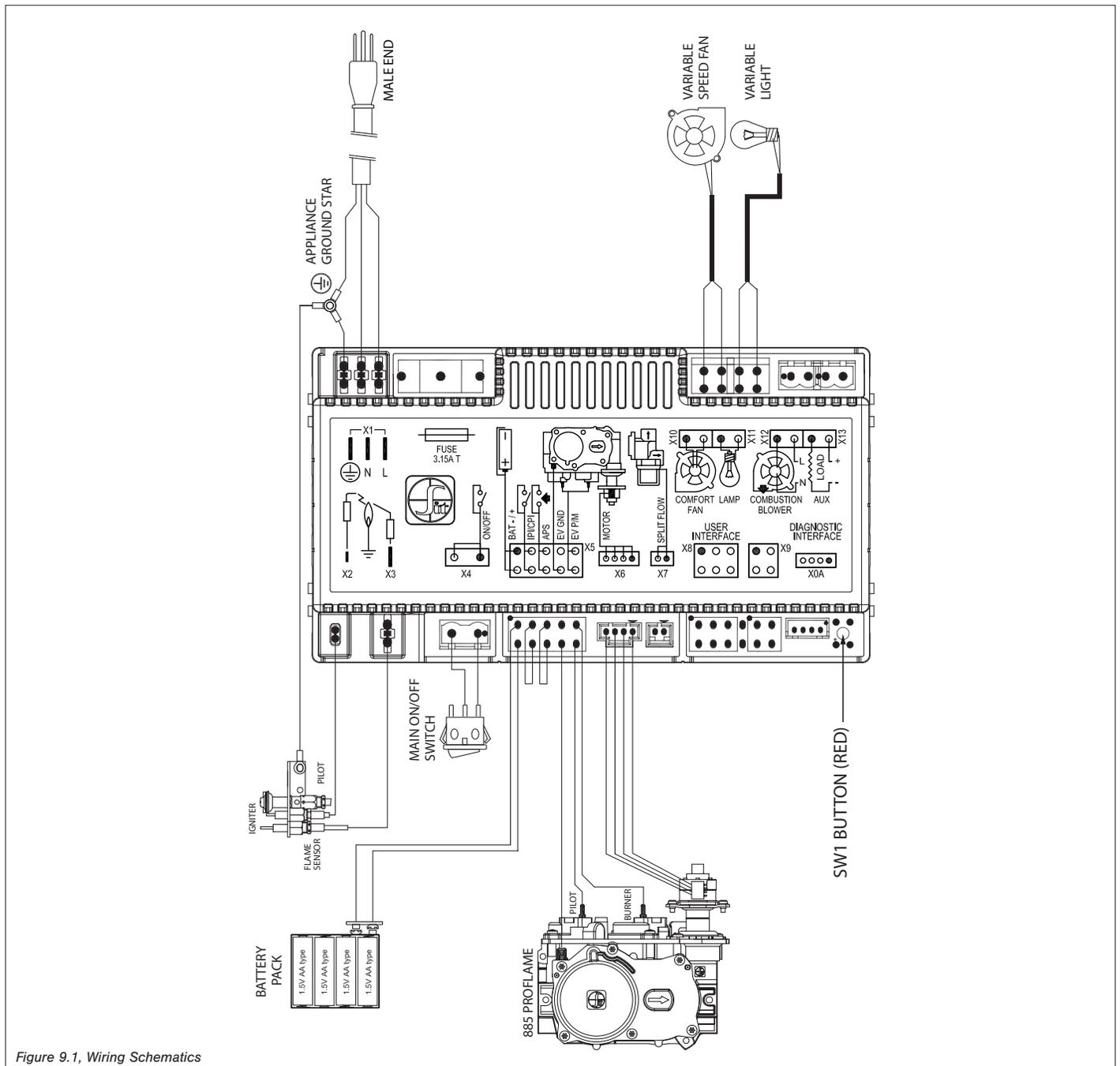
Figure 9.1, Wiring Schematics
