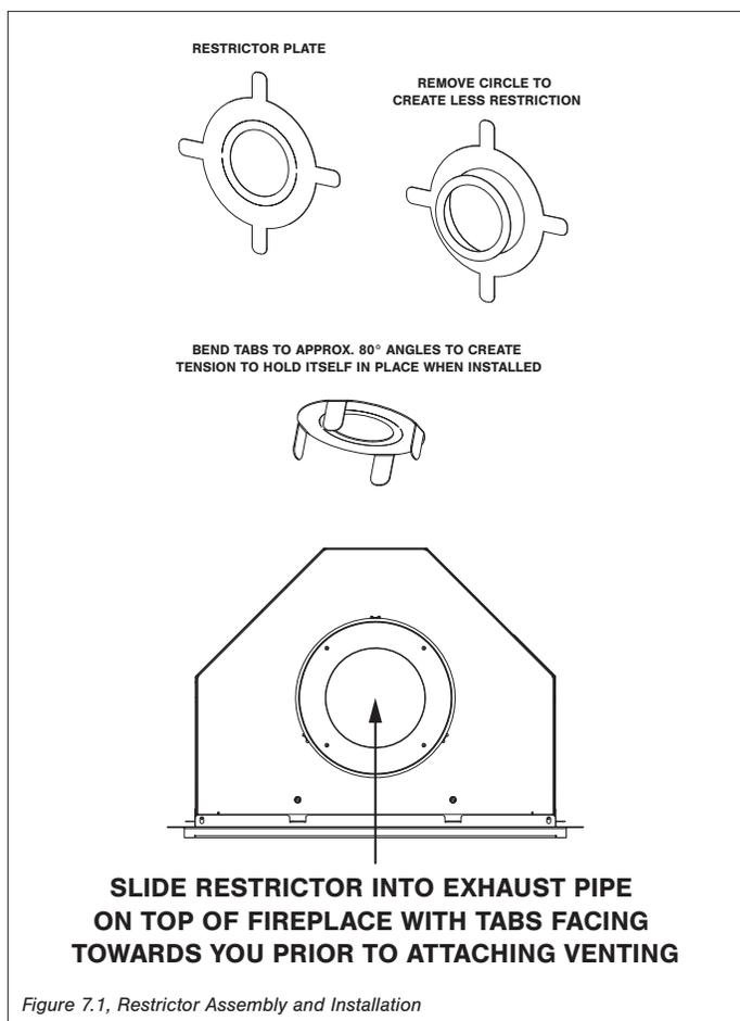
Figure 7.1, Restrictor Assembly and Installation
