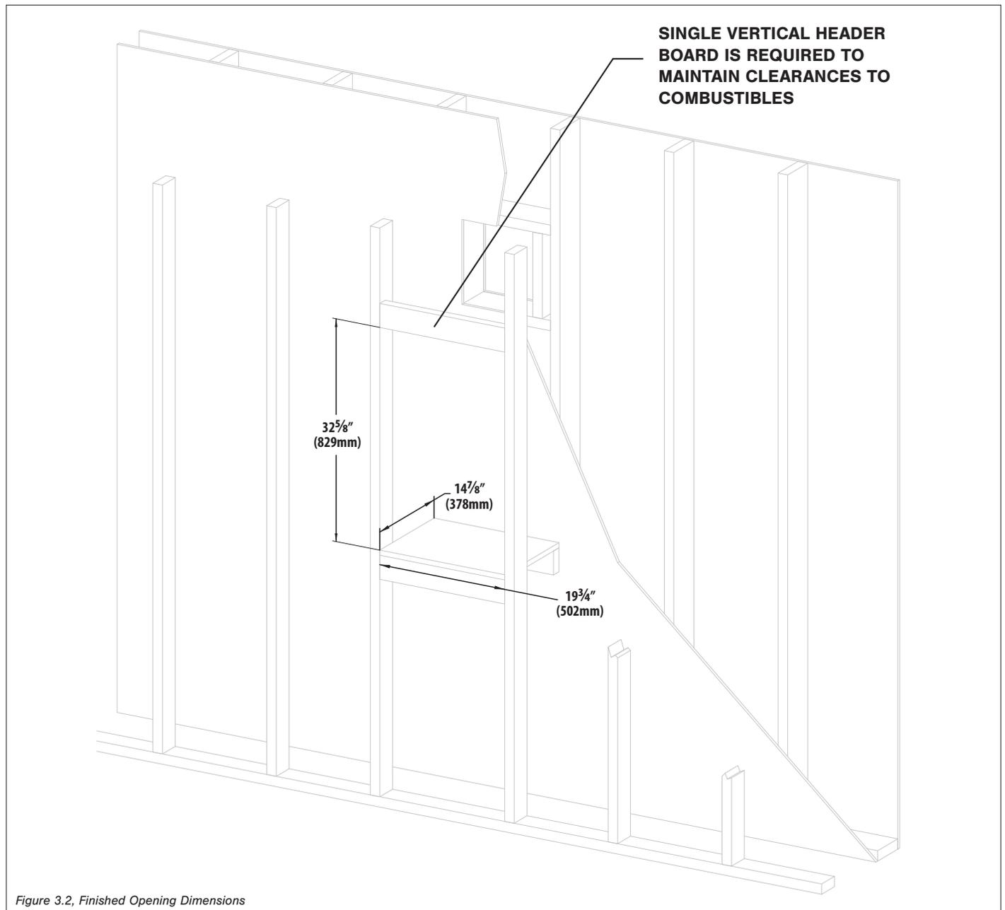
Figure 3.2, Finished Opening Dimensions
