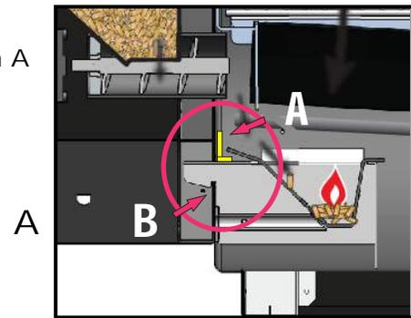
Install the Burn Grate Diagram B
