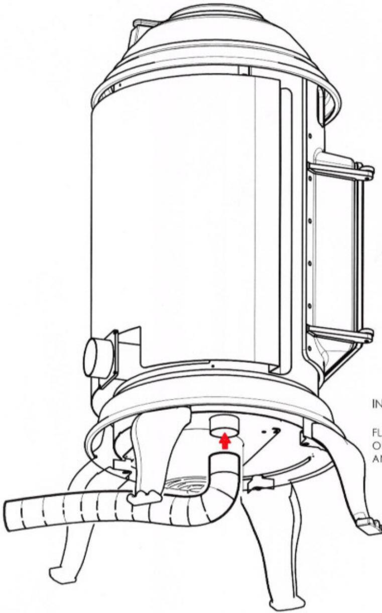
INSTALLING THE OUTSIDE AIR INTAKE TUBE.
